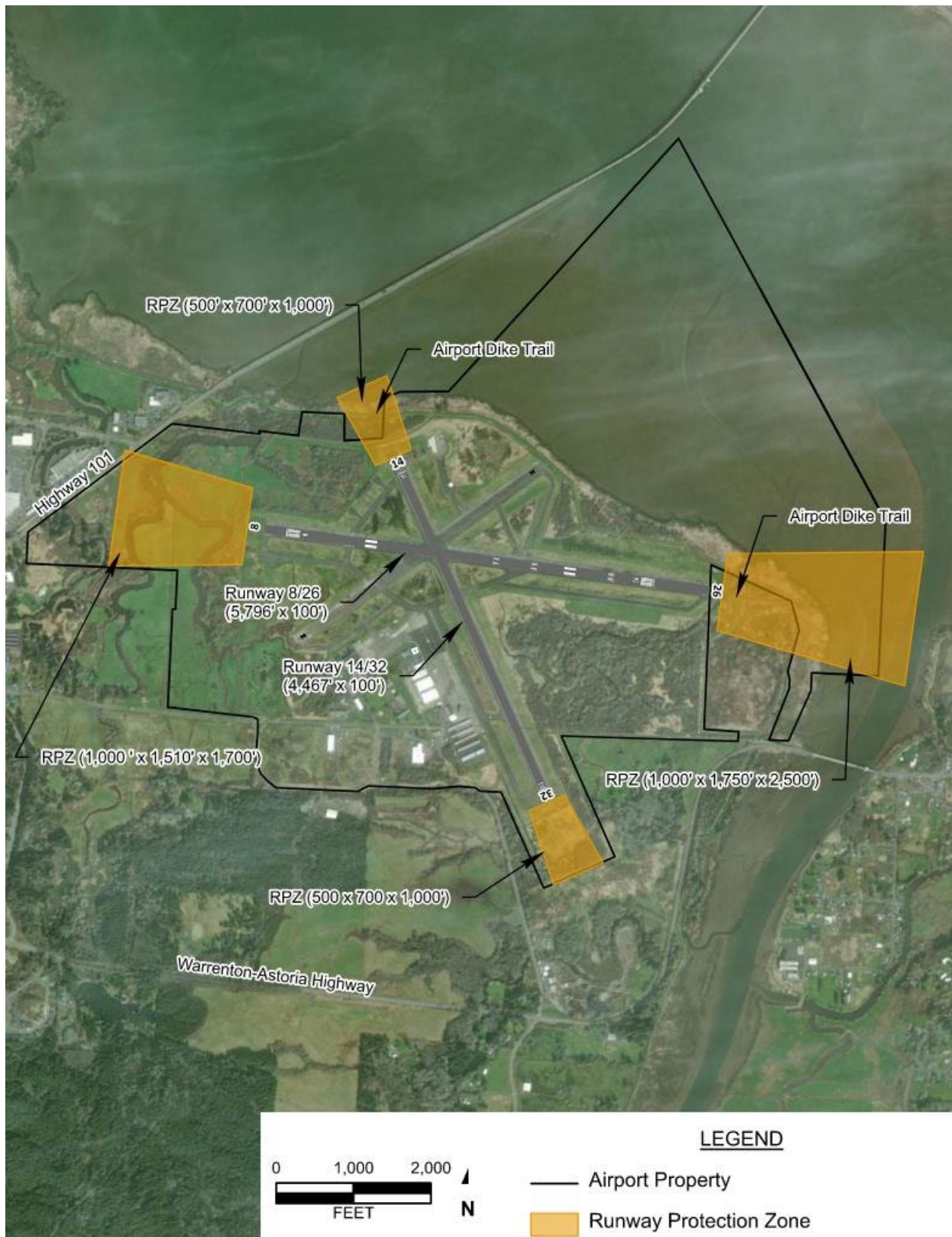
Figure 7-7: AST Runway Protection Zones (RPZs)
