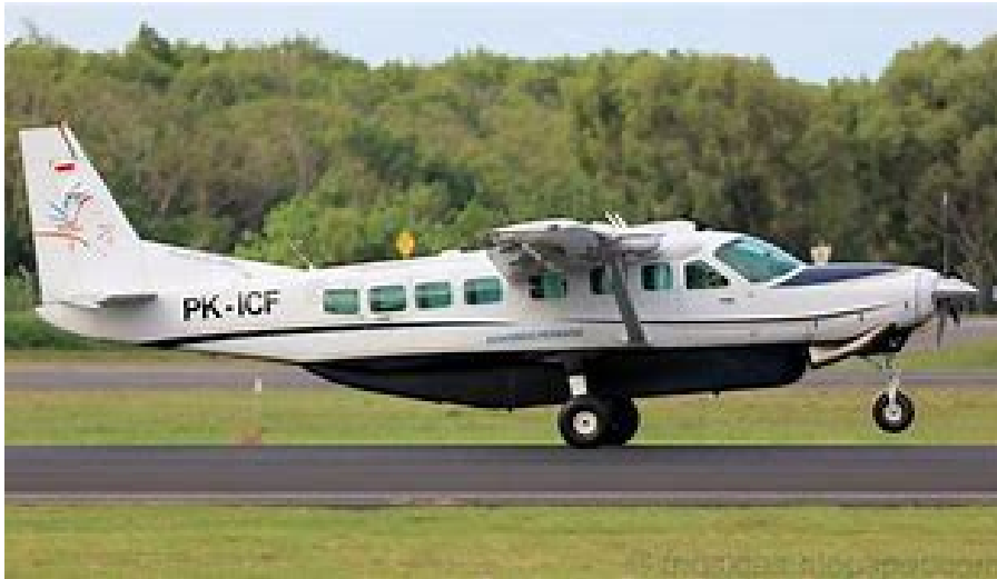
Figure 3-11: ARC B-II Representative Aircraft: C208 – Cessna 208 Caravan
