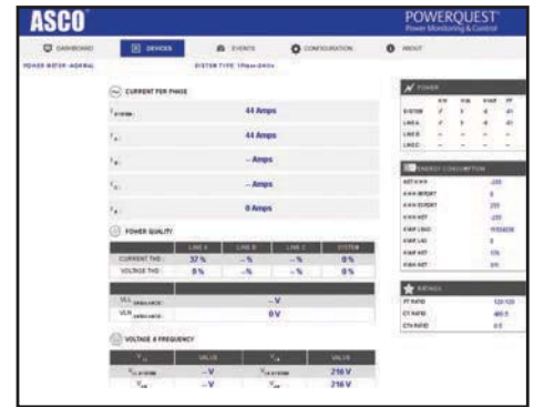
Fig. 18: Power Metering Screen
